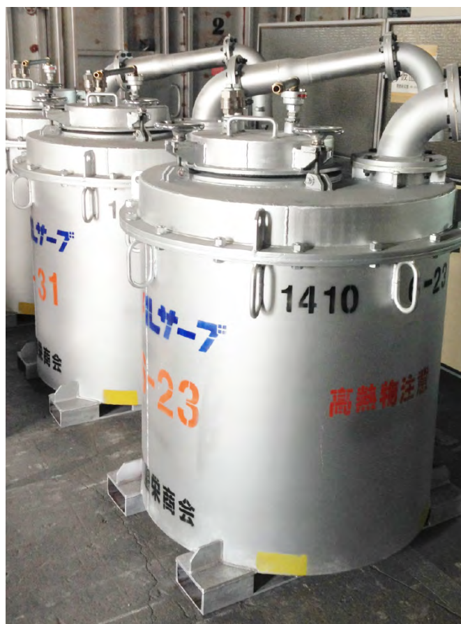
Filling of transfer ladle generates an average of 5.2 kg/Ton of oxides with standard pouring system, down to 0.9 kg/Ton with Al Serve vacuuming system.
